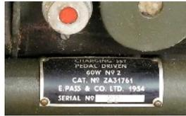
Close-up view of type and serial number plate apparently missing the 'Mk.1' notation as the No. 2 had not a charging indicator lamp.
